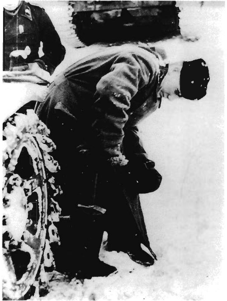
A heavily clad soldier of “Totenkopf” works on the track of a Sturmgeschütz III. The man pictured was probably a member of the Werkstattzug of the Division’s Sturmgeschütz Abteilung. The Germans were often able to salvage and repair damaged vehicles in the field, returning them quickly to action. The Russians did not have the same capability in the first years of the war because they generally lacked anything more than rudimentary repair facilities, although the Russian tankers themselves often found ingenious ways to keep their tanks running. (Credit National Archives)
