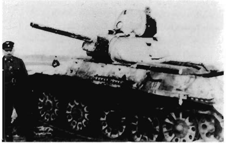
An early model Soviet T-34. The T-34, although a robust and durable tank with good sloped frontal armor and an adequate gun, had several design flaws. The tank commander had to help operate the gun and could not devote his entire attention to the command of the tank. In addition, the absence of a turret cupola hindered the ability of the commander to see well. The most serious problem was the lack of a radio other than those of the company or battalion commander. This prevented individual tanks from communicating with each other and more critically, did not allow commanders to direct the tanks of their unit once combat began. In contrast, German tanks were equipped with radios and a tank commander could talk with each member of the crew and any other tank. (Credit National Archives)
