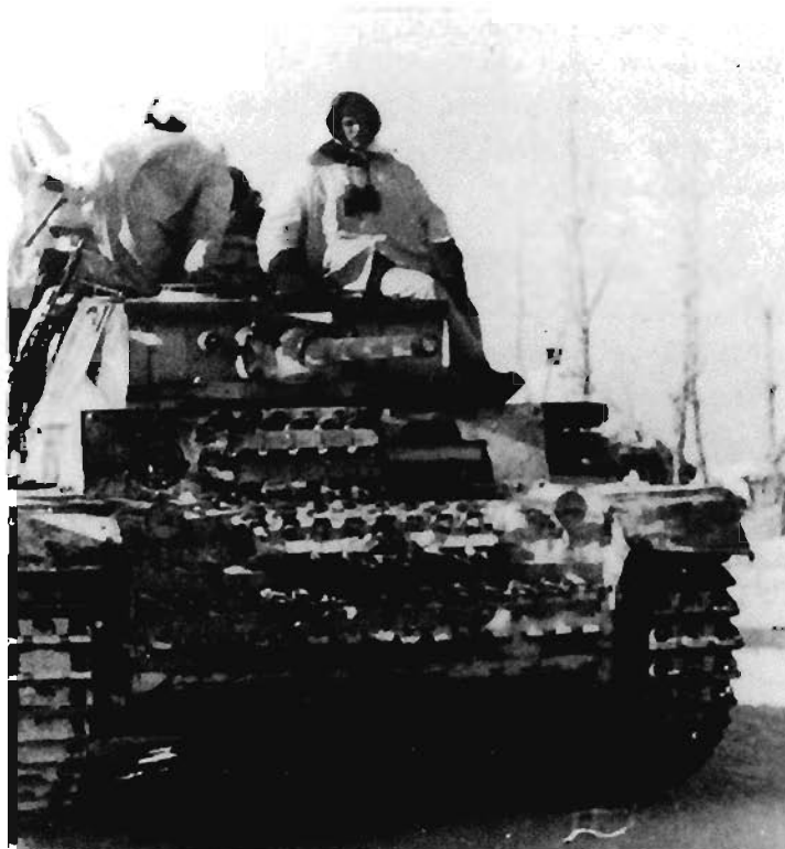
A Panzer III of SS-Panzer-Regiment 2 with several "Das Reich" Panzergrenadiers perched on its decks. When the division occupied defensive positions along the Oskul River in late January, the Panzer Regiment had 66 Panzer IIIs in its two battalions. It is armed with a 5cm cannon which was later upgraded with a longer barreled gun of the same caliber. The improved gun had a much greater shell velocity. (The author's collection)
