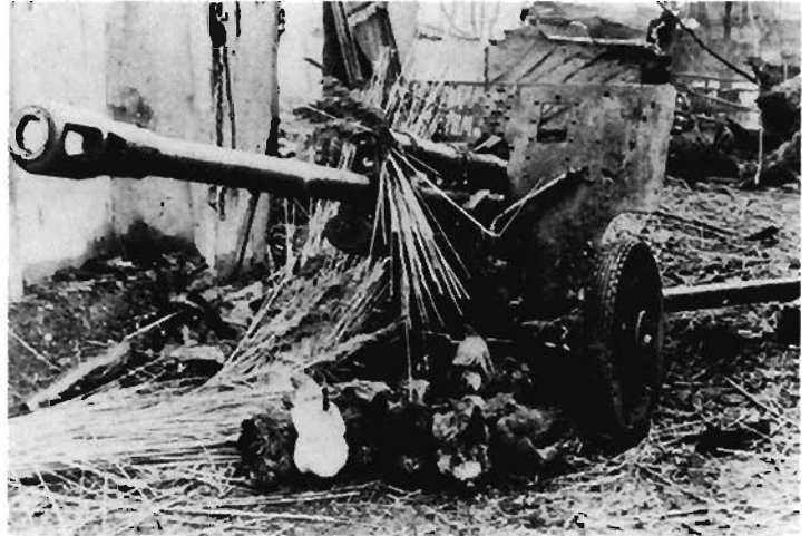
A good picture of a Russian 7.62 gun that has been abandoned in a village street and taken over by a number of chickens. The gun fired a high velocity anti-tank shell that could penetrate the frontal armor of the Panzer III and Panzer IV at ranges out to 800 to 1000 meters. It was designed as a light artillery piece and fired a high explosive shell also. (Credit National Archives)
