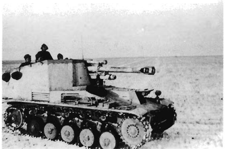
A self-propelled howitzer belonging to "Leibstandarte's" artillery regiment. This particular model was known as the "Wespe" and featured a 10cm light field howitzer mounted on a Panzer II chassis. The gun crew was protected by light armor in an open topped configuration. (Credit National Archives)
