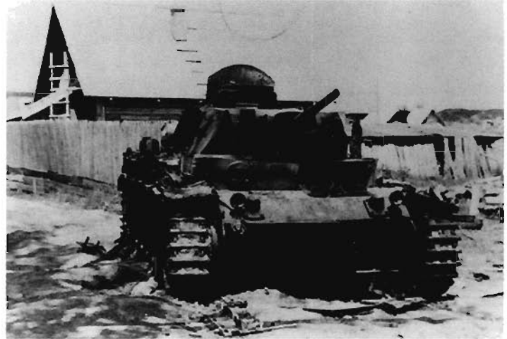
An SS Panzer III knocked out by two apparently tremendous impacts on both the frontal armor and the armor in front of the driver. The force of the explosions completely ruptured the steel plate and left gaping holes in the frontal armor of the tank. (Credit National Archives)
