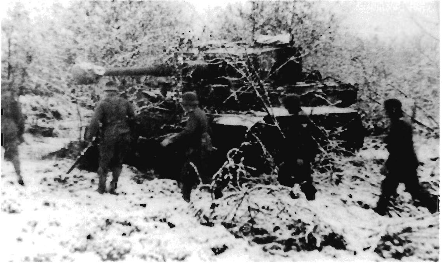
A disabled SS "Tiger" camouflaged with brush and snow. The 8.8 cm gun of the "Tiger" was very effective and could penetrate the frontal armor of any Soviet tank. However, there were limitations upon their use, particularly in the southern Ukraine, where bridges were often too weak to bear the weight of the huge tanks. The "Tiger" was also a more complex tank than the robust and simple Russian T-34. As a result, sometimes there were more of the heavy Panzers out of action due to mechanical problems than through combat damage. (Credit National Archives)
