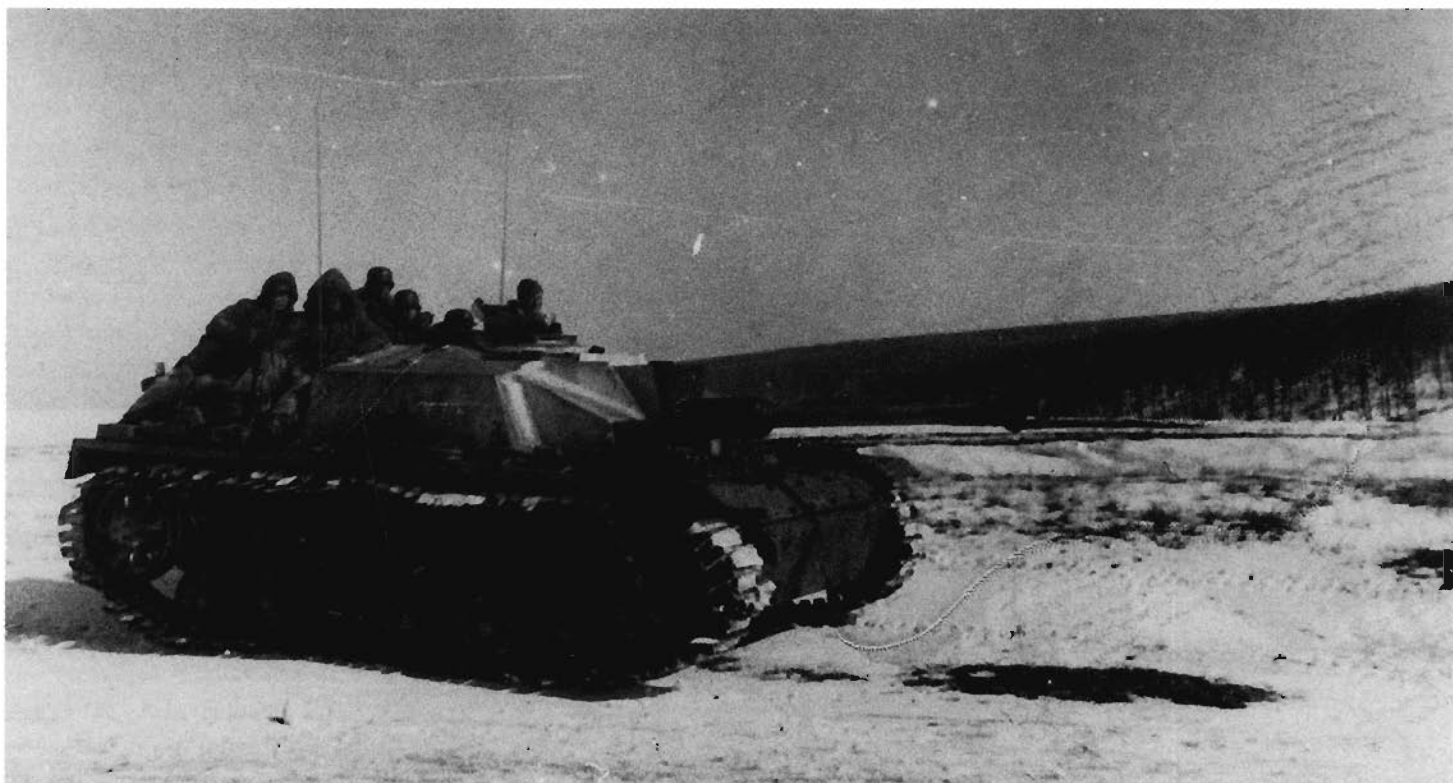
A "Das Reich" Sturmgeschütz III with the L48 main gun during early March of 1943. The L48 gun, which fired a high velocity 7.5cm round, replaced the original short barreled infantry gun. The assault guns were designed to furnish infantry support but gradually they became an important part of the anti-tank capability of the German divisions. (Courtesy Mark C. Yerger)
