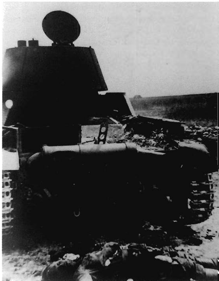
A Russian T-26 light tank with the armor covering its motor blown off by an internal explosion. The body of one of its crew lies behind the tank. The T-26 was used for reconnaissance and infantry support but was no match for even the up-gunned Panzer III. (Credit National Archives)
