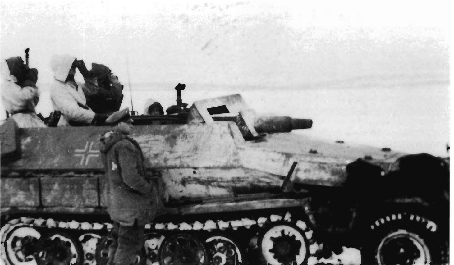
An SdKfz 251 with a 7.5cm short barreled infantry gun mounted in the space behind the driver. These vehicles and others equipped with a variety of heavy weapons furnished firepower for close support of the Panzergrenadier battalions (Credit National Archives)
