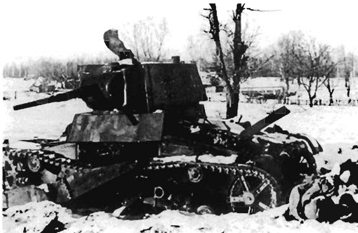
A knocked out Soviet T-70 light tank which appears to have suffered an internal explosion after being struck by a German shell. The T-70 was designed to be primarily an infantry support tank although it did not have a sufficiently heavy main gun to be more than marginally adequate in this role. It was lightly armored and the shells of Panzer IIIs and Panzer IVs could penetrate its frontal armor even at moderately long range. (Credit National Archives)
